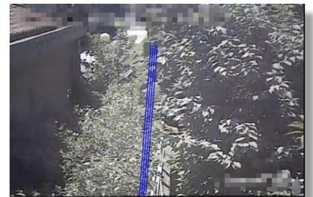
One customer sets line crossing rule on grass in a scene below, grass continuously makes false alarms which occupy DVR smart resource and storage space.
