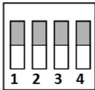
Figure 2. 1 DIP Switch Module (Binary Code: 0000)
