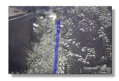
One customer sets line crossing rule on grass in a scene below, grass continuously makes false alarms which occupy DVR smart resource and storage space.
